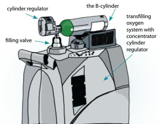
Transfilling Oxygen System With Concentrator Cylinder Regulator
